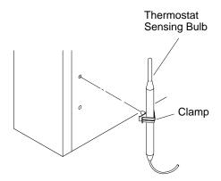
Figure 11 - Attaching Thermostat Sensing Bulb
